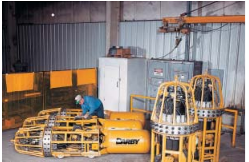
Final inspection before shipping Darby line-up clamps.
