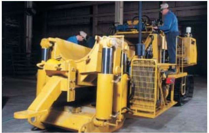
Darby workers fine-tune one of the first Series 2000 pipe benders to roll off the line.
