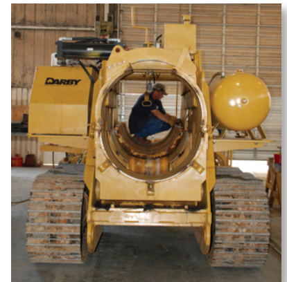
A Darby bending machine being prepared for the next job.
