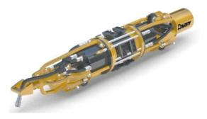
8" (203mm) Pipe Size Range Wall Thickness Range .125"-.375" (3.18-9.5mm) Standard Length 48" (1219mm) Width 8" (203mm) Height 8" (203mm) Weight 125 lbs (57 kg) Working Air Pressure 180-220 psi Air Motor Non Powered Air Tank .5 gal Clamping Shoes 10 total clamp shoes, 5 on each section Cylinder 5" (127mm) Climbing Capability N/A
